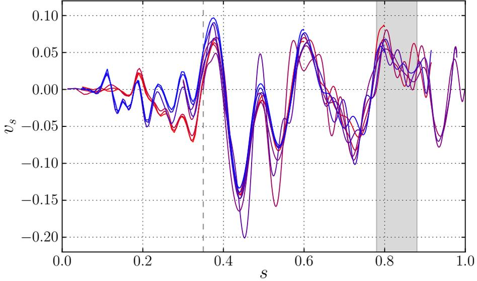
Figure 5: Velocity profiles ( $u_s$ ) as a function of cylindrical radius for different fixed height ( $-0.8 \leq z \leq 0.8$  with steps of 0.2, from blue to red) after  $366 T_\Omega$ , and at  $\phi = 0^\circ$  for case A. The shaded area indicates the location of the main torsional wave, and the velocities are in units of  $r_o \Delta \Omega / 1000$ .
