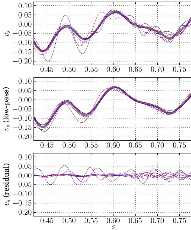
Figure 6: The data of figure 5 in the range  $s \in [0.42, 0.78]$  (top), after filtering out the scales smaller than 0.08 (middle), and the residual small scales (bottom). The bold grey curve is a  $z$ -average excluding the two most differing curves. Most of the departure from QG is contained in the small scales.
