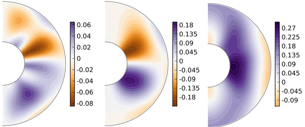
Figure 1: Meridional cross-section of the imposed magnetic field, in  $\max(|\mathbf{B}_0|)$  units. From left to right the cylindrical components  $(s, \phi, z)$  of the magnetic field at  $\phi = 25^\circ$ .
