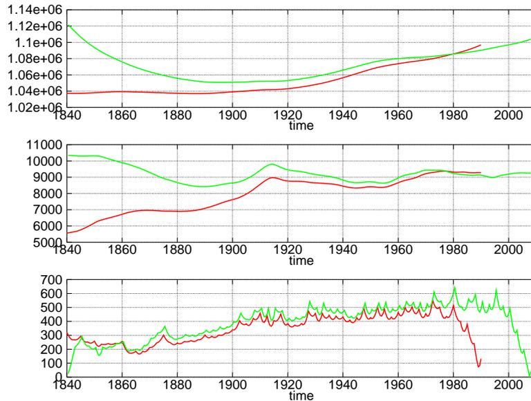
Figure C.15: From top to bottom: Magnetic Field (nT), Secular Variation (nT/y) and Secular Acceleration (right, nT/y<sup>2</sup>) norms for the model used in this study (green) and *gufm1* (red).
