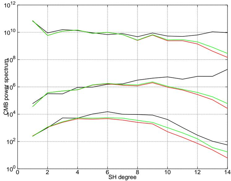
Figure C.14: From top to bottom: MF ( $\text{nT}^2$ ), SV ( $\text{nT}^2/\text{y}^2$ ) and SA (right,  $\text{nT}^2/\text{y}^4$ ) spectra, time averaged respectively over 1900–1980 for the model derived for this work (green) and *gufm1* (red), and over 2000–2006 for xCHAOS (black).
