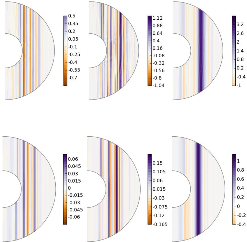
Figure 3: Meridional cross-sections of the velocity field. From left to right: the non-axisymmetric components of the velocity field  $u_s$  (cylindrical radial) and  $u_\phi$  (azimuthal) at  $\phi = 25^\circ$ ; and the axisymmetric component  $u_\phi^{m=0}$ . Velocities are in units of  $r_o \Delta \Omega / 1000$ . Top : case A at  $t = 183 T_\Omega$  after the impulse. Bottom : case B at  $t = 366 T_\Omega$  after the impulse.
