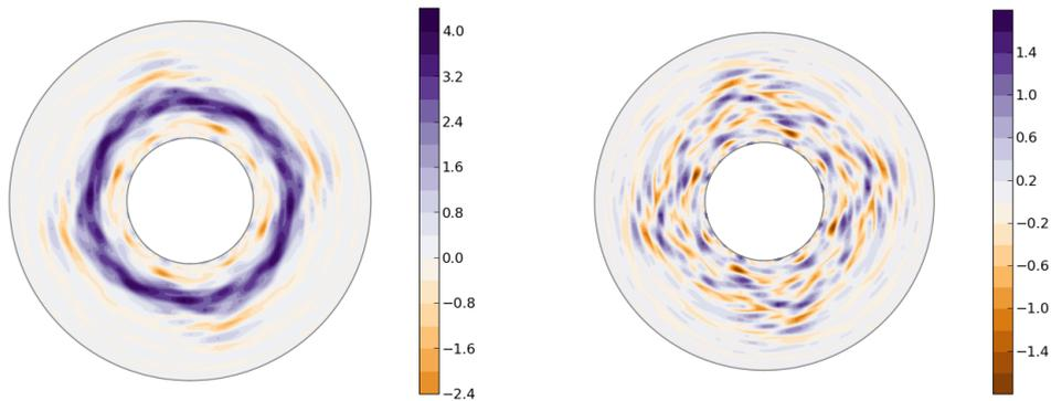
Figure 2: Equatorial cross-section of azimuthal component of the total (left) and non-axisymmetric (right) velocity field  $u_\phi$  at  $t = 183 T_\Omega$  after the impulse (case A). The velocities are in units of  $r_o \Delta \Omega / 1000$ .
