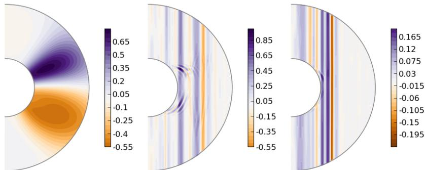
Figure 4: Meridional cross-section at  $\phi = 0^\circ$ , where the magnetic field almost reaches its strongest intensity. Left: cylindrical radial component of the imposed magnetic field. Middle to right, cylindrical radial component  $u_s$  for cases A and B, respectively at  $t = 183 T_\Omega$  and  $t = 366 T_\Omega$  after the impulse. The magnetic field is in  $\max(|\mathbf{B}_0|)$  units. Velocities are in units of  $r_o \Delta\Omega/1000$ .
