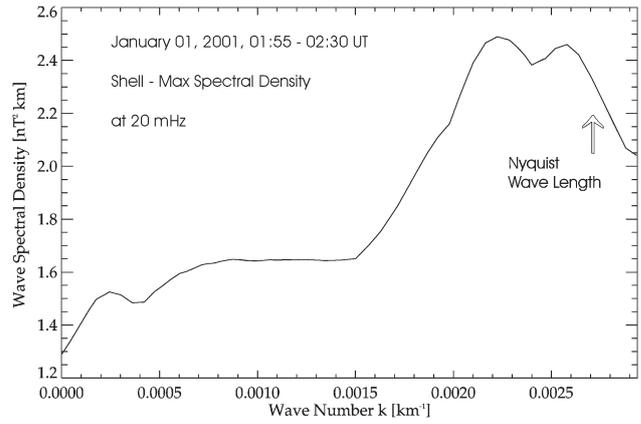
**Fig. 5.** Shell-max spatial spectral density distribution in logarithmic representation resulting from applying the wave telescope to measurements in the magnetosheath during the interval 1 January 2001, 01:55–02:30 UT.
