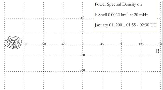
**Fig. 6.** Spectral density distribution on the  $k$ -shell  $k = 0.0022 \text{ km}^{-1}$  resulting from applying the wave telescope to measurements in the magnetosheath during the interval 1 January 2001, 01:55–02:30 UT. The logarithm of the power is displayed. ‘B’ denotes the position of the mean magnetic field direction.
