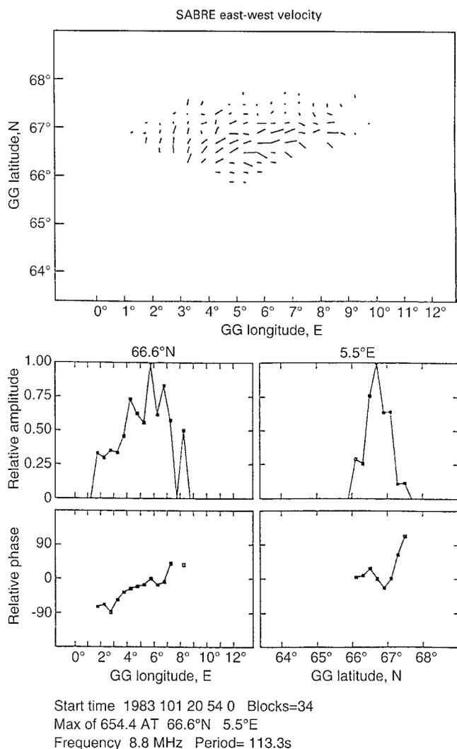
**Fig. 7.** Amplitude and phase characteristics throughout the SABRE field of view (*top*) determined from FFT spectral analysis of the SABRE east-west velocity component data on day 101, 1983. The amplitude (*middle*) and phase (*bottom*) as a function of latitude are very complicated around the amplitude peak while the longitudinal phase difference of  $\sim 50^\circ$  in  $\sim 3^\circ$  of longitude implies an  $m$  value of  $\sim 17$  and a westward propagating wave
