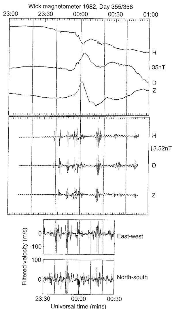
**Fig. 4.** Time series data for the event on day 355/356 1982. From *top to bottom* of the figure, unfiltered and filtered ground magnetometer data from the only operational BGS station at this time (Wick) are presented together with filtered SABRE east-west and north-south velocity component data
