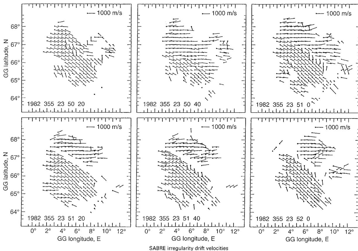
**Fig. 5.** A sequence of 20 s resolution SABRE spatial velocity plots from day 355, 1982 at the time of the second Pi2 pulsation where a region of strongly eastward velocity replaces the south-eastward
