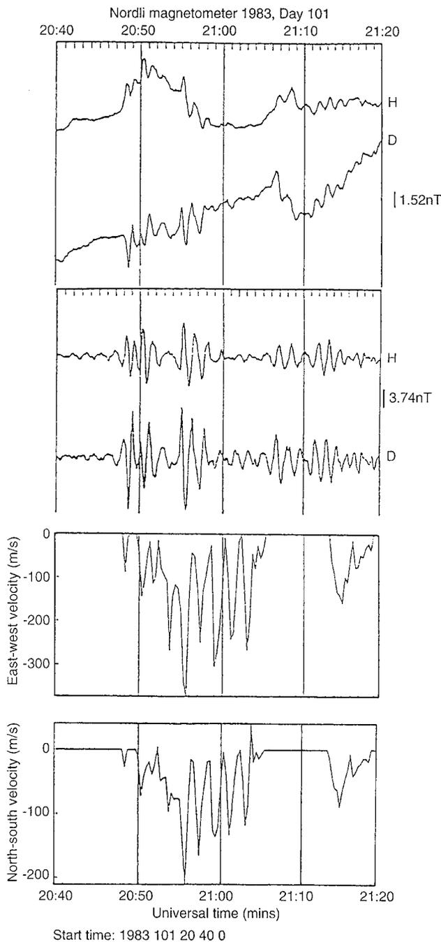
**Fig. 6.** Time series data for the Pi2 pulsations present on day 101, 1983. From *top to bottom*, unfiltered and filtered ground magnetometer data from Nordli are presented together with SABRE east-west and north-south velocity component data. The SABRE data were averaged over the small region of backscatter present during the event, from  $66^\circ$  to  $67.6^\circ\text{N}$  and  $4^\circ$  at  $6^\circ\text{E}$
