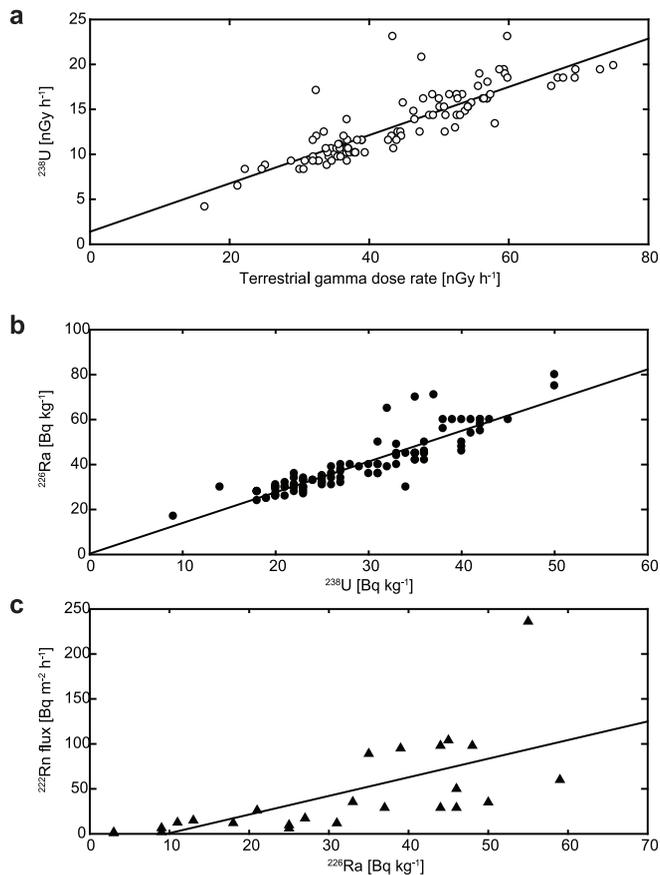
**Fig. 1.** Correlations between (a) the contribution of GDR originating from the  $^{238}\text{U}$  decay series and total terrestrial gamma dose rate; (b)  $^{226}\text{Ra}$  activity and  $^{238}\text{U}$  activity and (c)  $^{222}\text{Rn}$  flux at the soil surface and soil  $^{226}\text{Ra}$  activity. Data for (a) and (b) was kindly provided by SUER (Section of Surveillance of Radioactivity, Switzerland).
