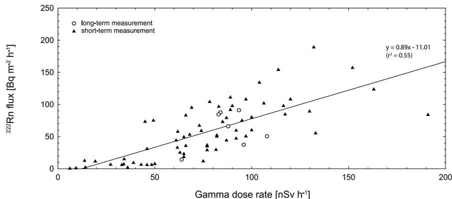
**Fig. 2.** Correlation of  $^{222}\text{Rn}$  flux and terrestrial gamma dose rate measured at field sites in Switzerland, Germany, Scotland, Finland and Hungary.
