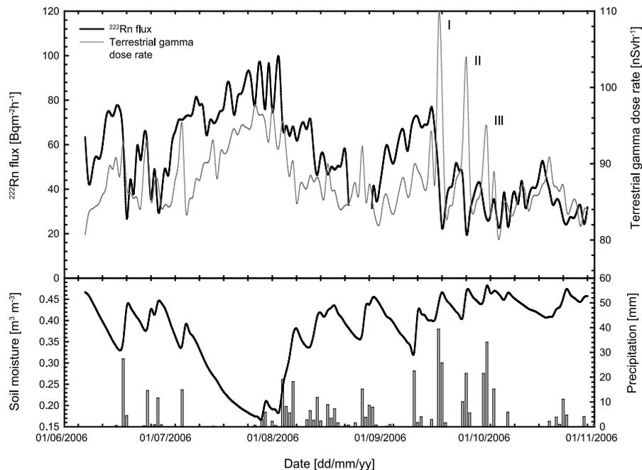
**Fig. 3.**  $^{222}\text{Rn}$  flux, terrestrial gamma dose rate, precipitation and soil moisture time series from June to November 2006 in Basel (Switzerland). Heavy rain events are marked with I, II and III.
