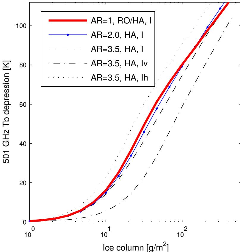
**Fig. 5.** Relationship between 501 GHz  $T_b$  depression and cloud ice amount, for different assumptions on particle shape and orientation where: AR = aspect ratio, RO = randomly oriented, HA = horizontally aligned, I = mean of  $I_v$  and  $I_h$ , and  $I_{v/h}$  = intensity at vertical and horizontal polarisation, respectively. Simulations for MH97 PSD and cloud ice between 12 and 14 km.
