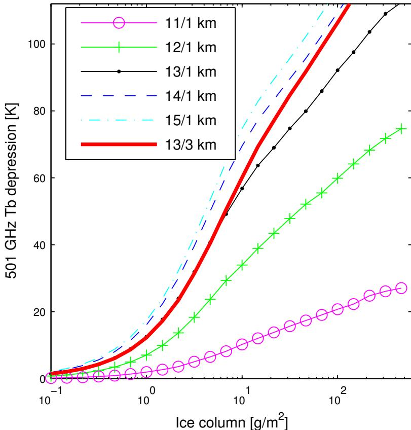
**Fig. 6.** Relationship between 501 GHz  $T_b$  depression and cloud ice amount, for different cloud altitudes and layer thicknesses. For example, the dotted line is for a cloud centre altitude of 13 km and a 1 km thick cloud layer. Simulations for 7 km tangent altitude and the 200  $\mu\text{m}$  gamma distribution.
