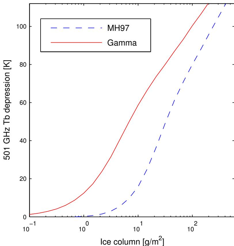
**Fig. 4.** Relationship between  $T_b$  depression and cloud ice amount, for two different particle size distributions. Simulations for 501 GHz, 7 km tangent altitude and cloud ice between 12 and 14 km.
