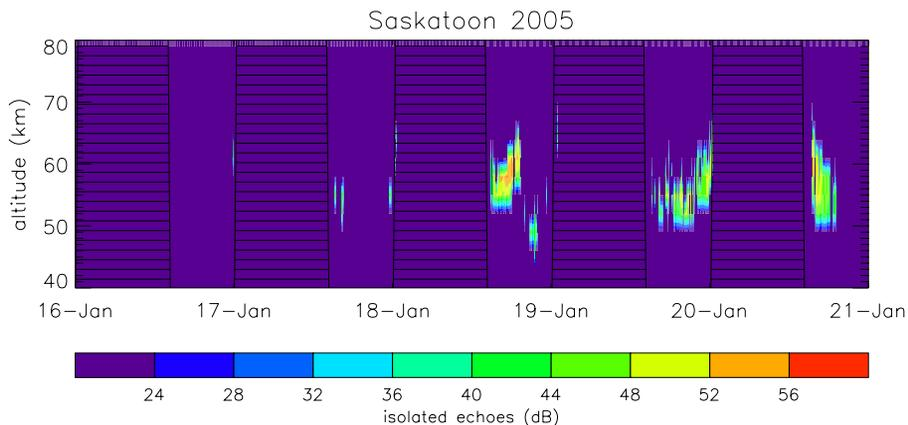
**Fig. 4.** Sequence (16–21 January 2005) of ILME seen by the Saskatoon MFR ( $52^{\circ}$  N), corresponding to the upper panel of Fig. 2. Note that the date axis is in UT and corresponds to that in Fig. 2, such that daylight hours occur some 7 h later relative to Tromsø.
