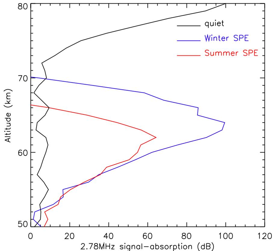
**Fig. 7.** Schematic illustrating conceivable profiles of MF radar returns. The black solid line shows a power profile from a quiet ionosphere with no non-deviative absorption present. The red and blue lines indicate echo power from the same electron density profile during a solar proton event (SPE), but with summer and winter non-deviative absorption taken into account.
