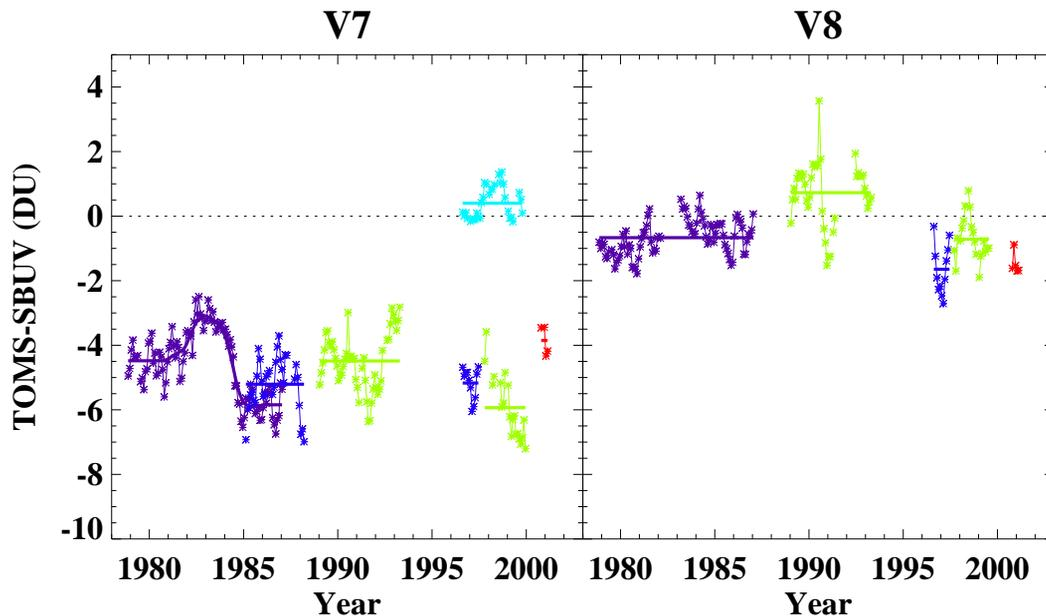
**Fig. 3.** The two panels show the inter-instrument comparisons (TOMS-SBUV) for all available overlap periods plotted as a function of time. Version 7 data are shown in the left panel and version 8 data in the right panel. The plotted differences are averaged from 50° N–50° S. We use these differences to determine the best offsets to apply to each data set in order to create an internally consistent calibration for the MOD data set.
