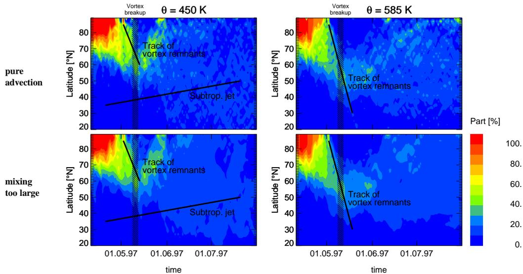
**Fig. 5.** Meridional (zonally averaged) contribution of vortex air at  $\theta = 450$  (left) and  $585$  K (right) for CLaMS simulation without (top) and with excessive (bottom) mixing. The colors denote the zonally averaged rate the vortex air changing from 100% (pure vortex air) to 0% (pure extra vortex air). The black lines denote the tracks of the vortex air masses during their transport into the mid latitudes (see also Fig. 4).
