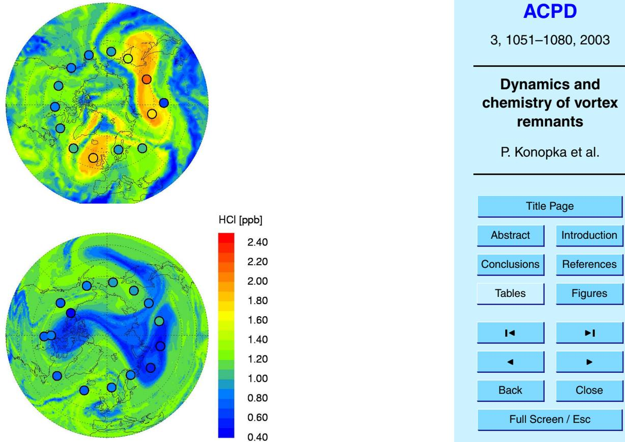
**Fig. 8.** HCl simulated with CLaMS at  $\theta = 450\text{K}$  2 days after the vortex breakup at 12 May 1997 (top) and 17 March 2000 (bottom). High values of HCl indicate a completed chlorine deactivation. The circles denote the HALOE observations.
