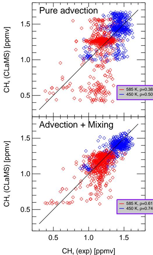
**Fig. 3.** CLaMS transport of CH<sub>4</sub> versus HALOE observations northward of 30° N between 10 April and 31 June 1997 at  $\theta = 450$  and  $\theta = 585$  K without mixing (upper panel) and with adjusted mixing (lower panel).
