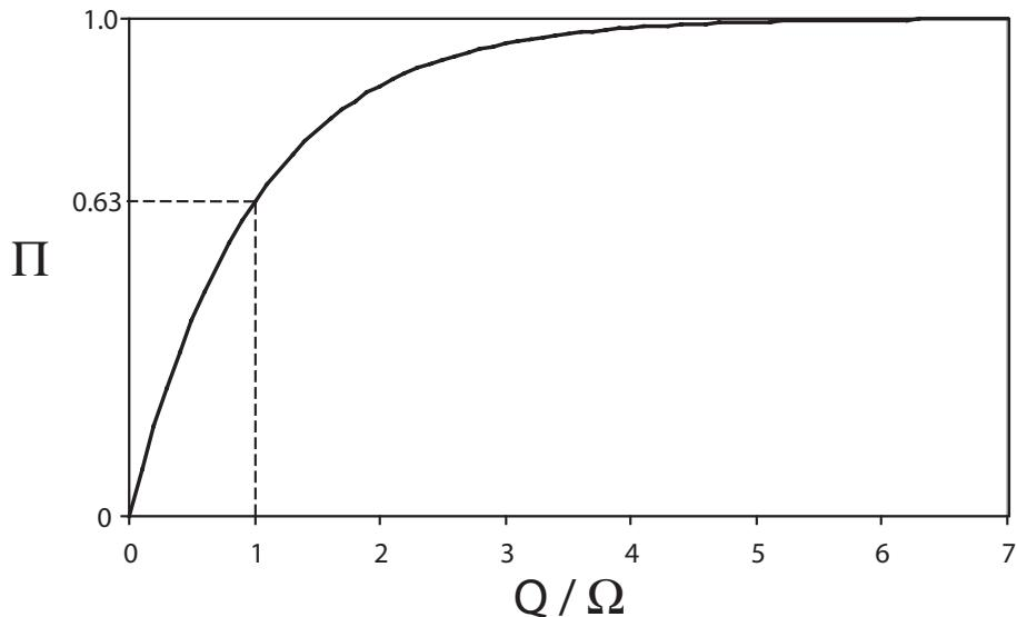
**Fig. 6.** A transfer function used in the model for estimating transport of dissolved P. When  $Q=\Omega$ , it is assumed that 63% of dissolved P in the “interactive zones” around the preferential pathways is transported.
