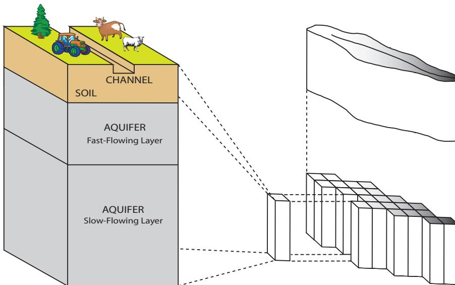
**Fig. 1.** Representation of a catchment in CAMEL. A catchment is represented using a network of square grid cells each of which represents the corresponding soil-aquifer column within the catchment. Based on this structure, the model simulates both surface and subsurface processes explicitly.
