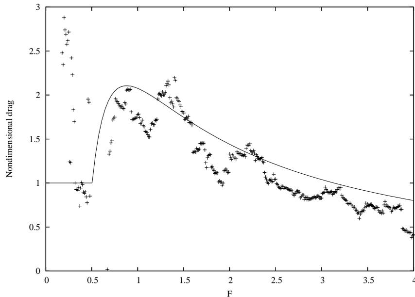
**Fig. 3.** The non-dimensional drag as a function of the inverse Froude number  $F$ . Solid line: theoretical dependency; crosses: diagnostic result from the pseudo-academic experiment over the Alps at the horizontal resolution of 10 km.
