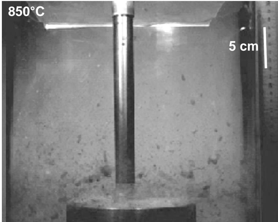
**Fig. 4.** Picture from a video of one 850°C impact experiment, showing total fragmentation of the rock sample. Note strongly horizontal directed movement of fine fragments (<http://www.electronic-earth-discuss.net/1/81/2006/eed-1-81-2006-supplement.zip>).
