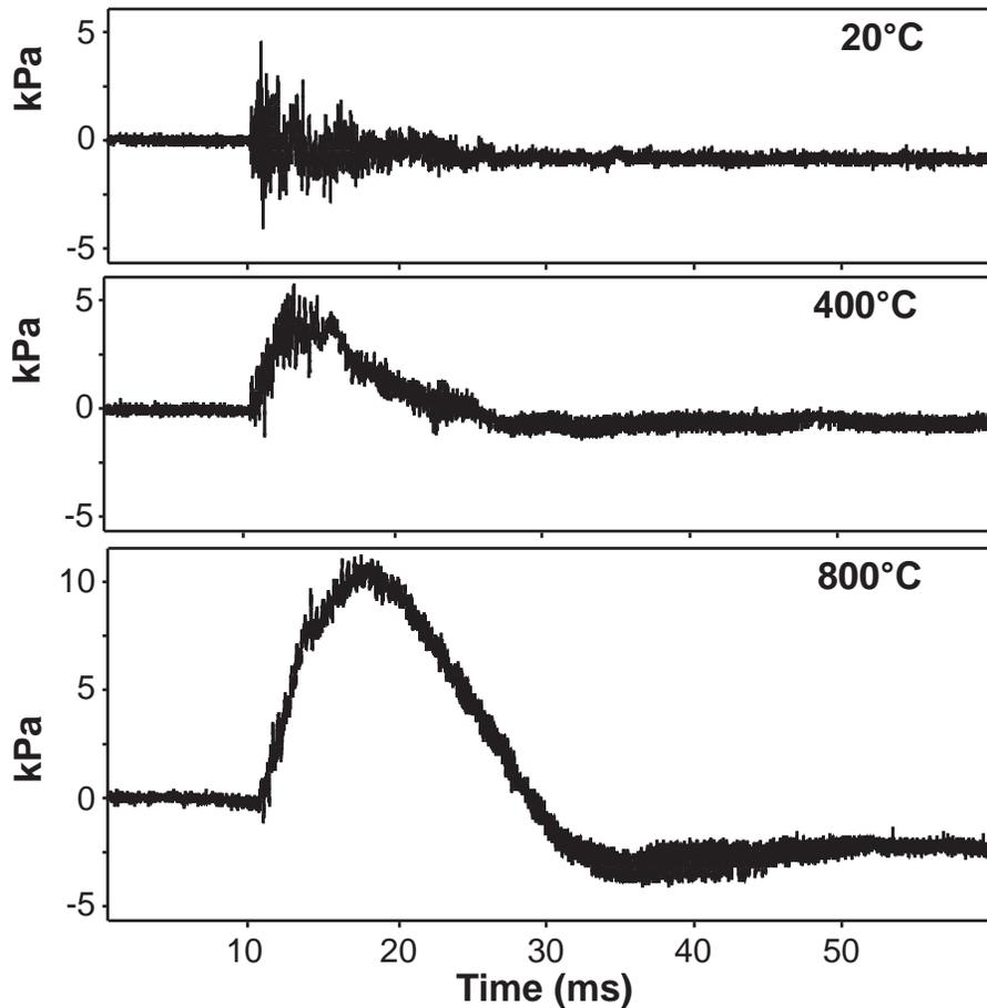
**Fig. 2.** Pressure data (kPa) from a pressure transducer located at the top of the impact section versus time (ms). Graphs show the pressure data from representative experiments at 20°, 400° and 800°C. Note sharply rising dynamic pressure waves occurring at higher temperatures.
