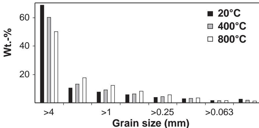
**Fig. 3.** Grain-size distributions of the fragments resulting from representative runs. Note significant decrease of the coarse and increase of the fine fractions strongly depending on sample temperatures.
