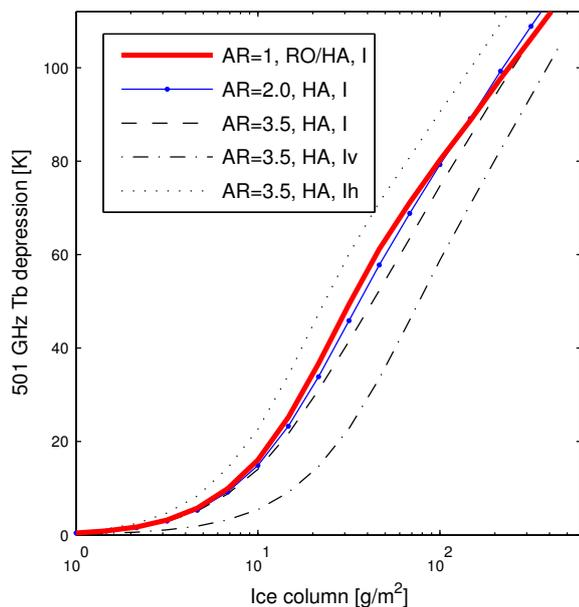
**Fig. 5.** The relationship between 501 GHz  $T_b$  depression and cloud ice amount for different assumptions on particle shape and orientation where: AR=aspect ratio, RO=randomly oriented, HA=horizontally aligned, I=mean of  $I_v$  and  $I_h$ , and  $I_v/h$ =intensity at vertical and horizontal polarisation, respectively. Simulations for MH97 PSD and cloud ice between 12 and 14 km.
