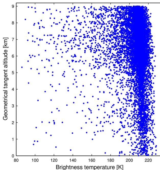
**Fig. 2.** Randomly selected values (10 000) from the 501 GHz part of the data set (mean over 501.2–501.3 GHz, all data from tropical latitudes). The band of data values around 210 K corresponds to clear-sky conditions and relatively thin clouds, while lower brightness temperatures can only be caused by more dense ice clouds.
