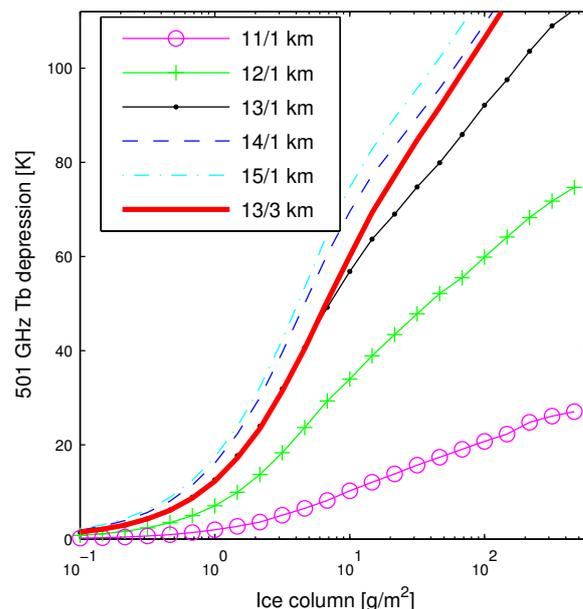
**Fig. 6.** The relationship between 501 GHz  $T_b$  depression and cloud ice amount for different cloud altitudes and layer thicknesses. For example, the dotted line is for a cloud centre altitude of 13 km and a 1 km thick cloud layer. Simulations are for 7 km tangent altitude and the 200  $\mu\text{m}$  gamma distribution.
