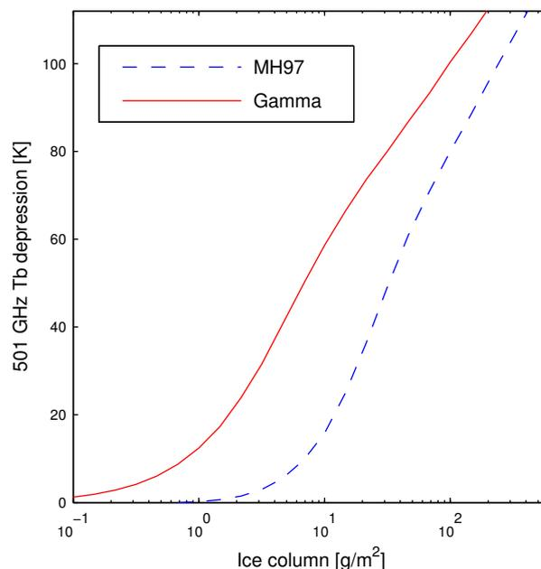
**Fig. 4.** The relationship between  $T_b$  depression and cloud ice amount for two different particle size distributions. Simulations are for 501 GHz, 7 km tangent altitude and cloud ice between 12 and 14 km.
