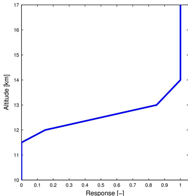
**Fig. 8.** Estimated altitude variation of cloud ice retrieval response. Data from other sources should be weighted with this response before being compared to Odin-SMR results obtained by the retrieval algorithm described here.
